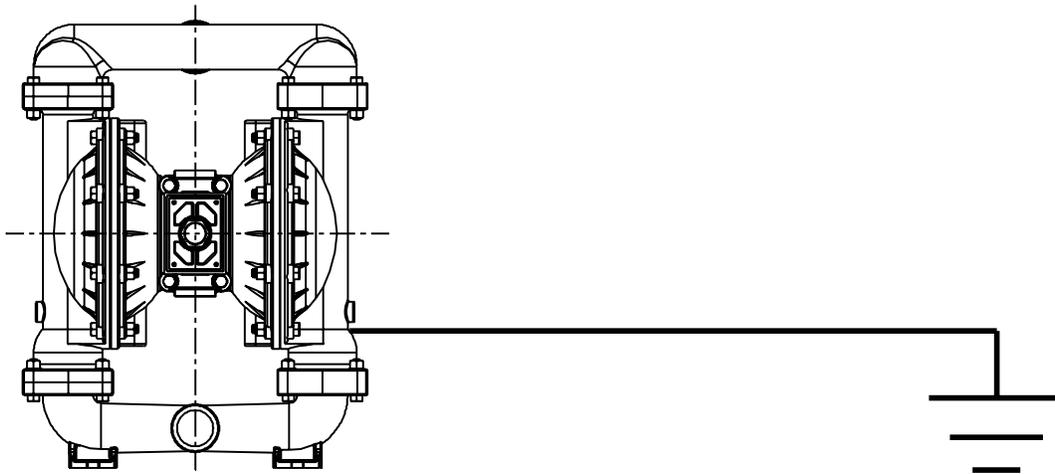
To reduce the risk of static electrical sparking, this pump must be grounded. Check the local electrical code for detailed grounding instruction and the type of equipment required, or in the absence of local codes, an industry or nationally recognized code having jurisdiction over specific installations.
