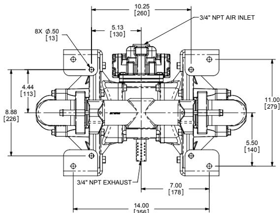
**2" NPT(F) Suction and Discharge • 3/4" NPT(F) Air Inlet
